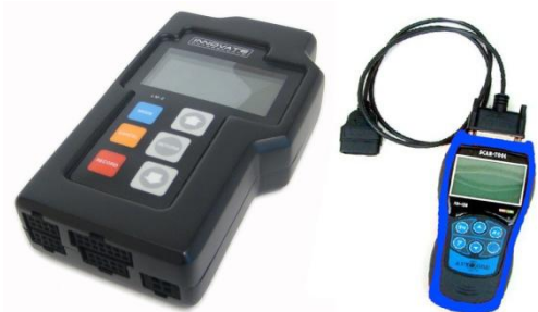
Picture no. 10 a: Hand testers: A) Wideband controller sensor B) OBD scanner
