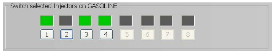
Picture no. 12b:Example – second injector works on gasoline
